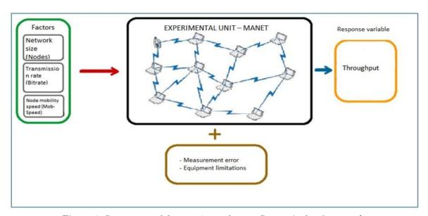
Figure 9. Components of the experimental setup. Source: Authors' own work.
