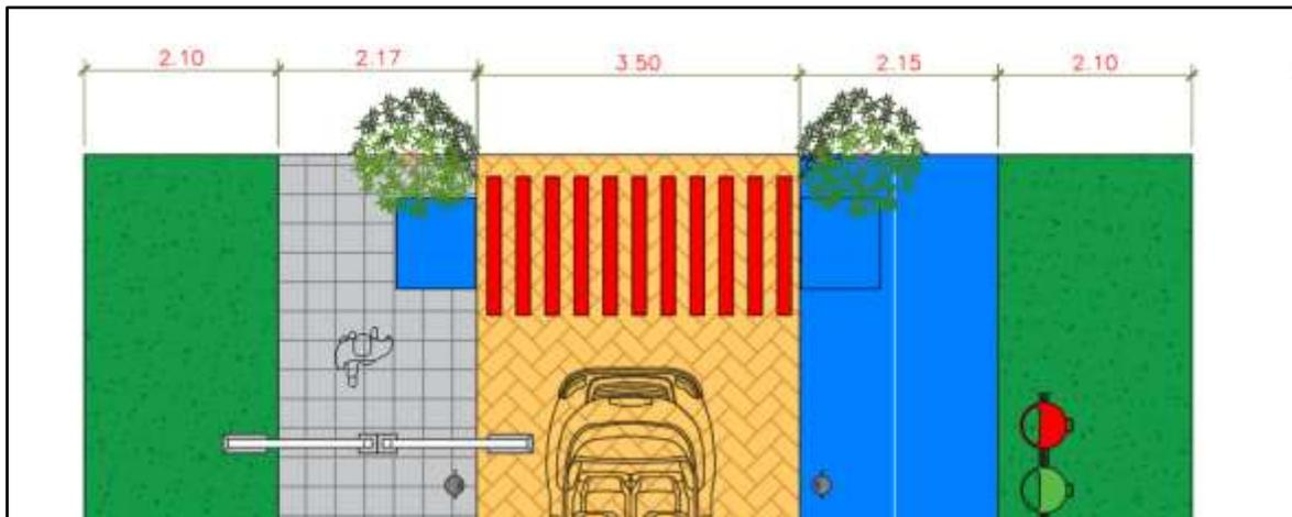
FIGURA 18 TRAMO PLANTA DISEÑO "PASO SOSTENIBLE" TRAMO PEATONAL Y CICLORRUTA.
